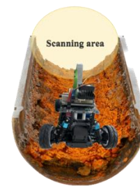
Figure 1 – Visualization of the pipeline scanning process for corrosion
