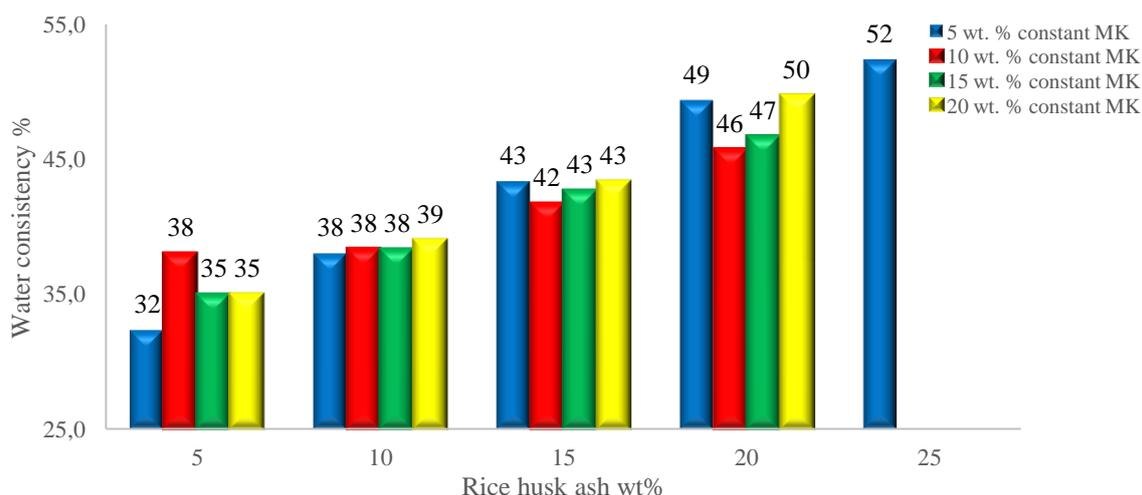
Figure 4 – Effect of RHA at constant MK on consistency of ternary blend
