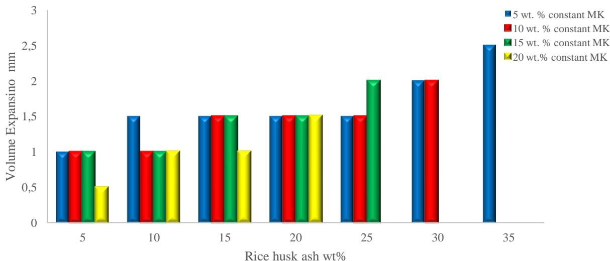
Figure 9 – Effect of RHA content at constant MK content on volume expansion of ternary blends
