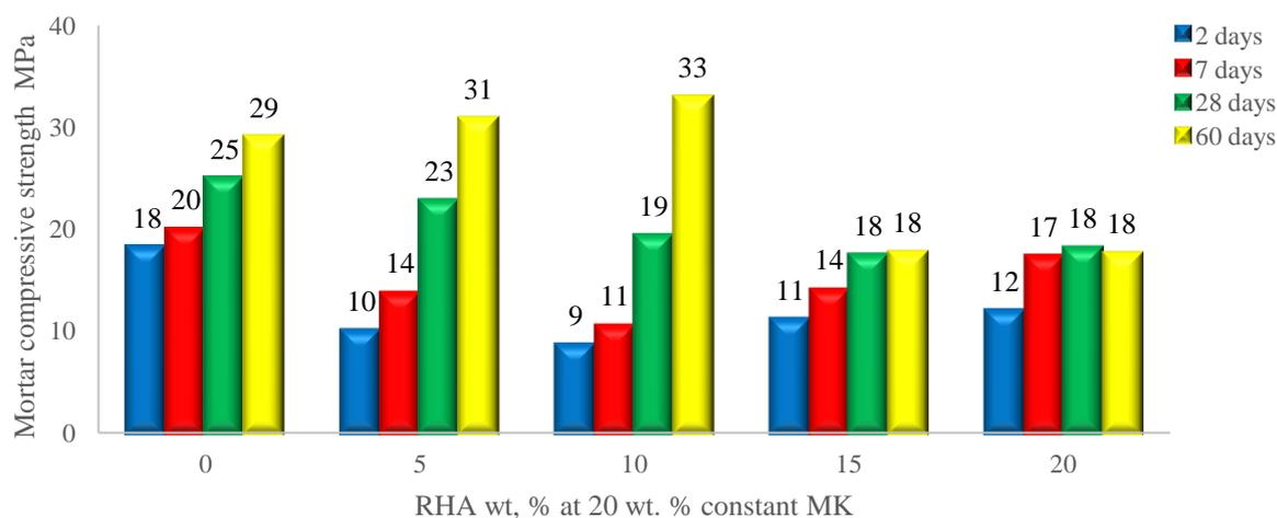
Figure 18 – Effect of RHA content at constant 20 wt% MK content on Strength of blends and OPC mortars
