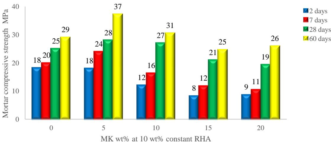
Figure 12 – Effect of MK content on mortar strength of blends at constant 10 wt% RHA and OPC
