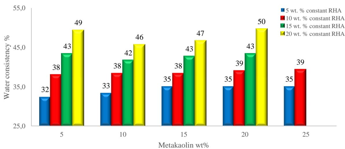
Figure 3 – Effect of MK at constant RHA on the consistency of ternary blend
