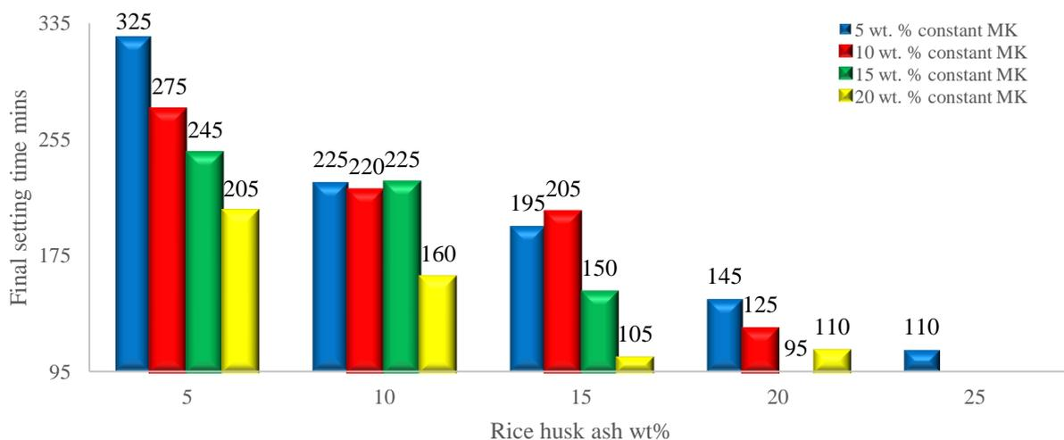
Figure 6 – Effect of RHA content at constant MK content on final setting time of ternary blends
