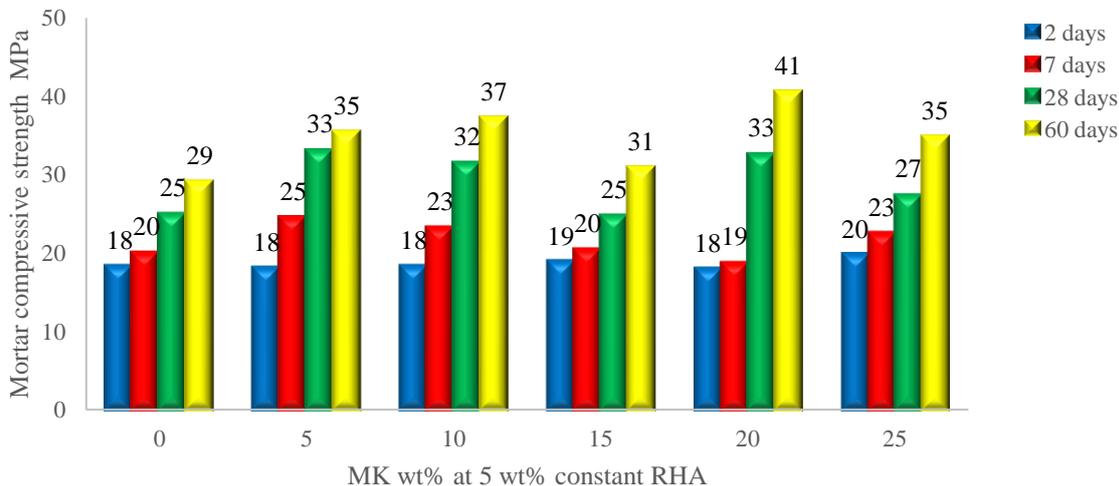
Figure 11 – Effect of MK content on Strength of blends and OPC mortars at 5 wt% constant RHA
