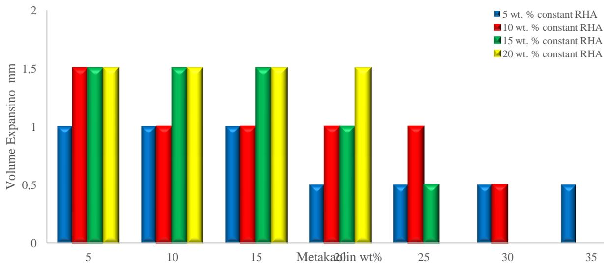
Figure 10 – Effect of MK content constant RHA content on volume expansion of ternary blends
