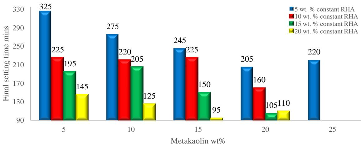
Figure 8 – Effect of MK content at constant RHA content on final setting time of ternary blends
