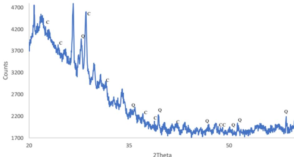
Figure 1 – X-ray Diffraction for RHA
