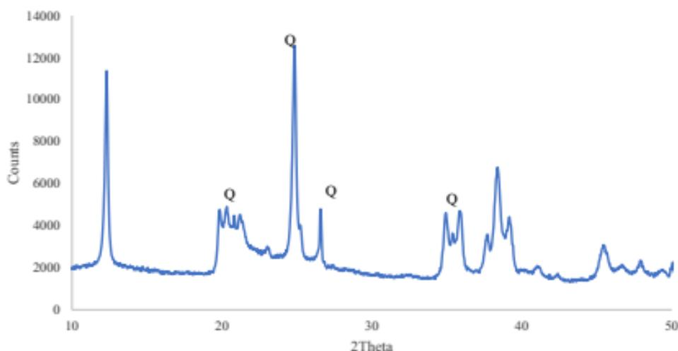
Figure 2 – X-ray diffraction for MK
