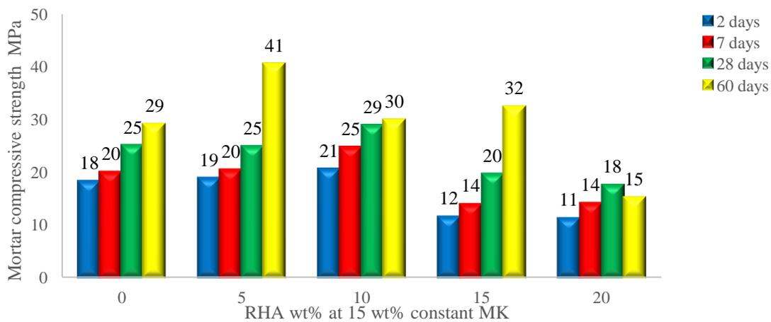
Figure 17 – Effect of RHA content at constant 15 wt% MK on compressive strength of blends and OPC mortars
