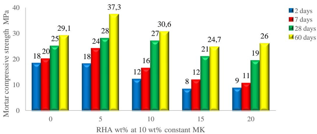
Figure 16 – Effect of RHA content at constant 10 wt% MK on compressive strength of blends and OPC mortars
