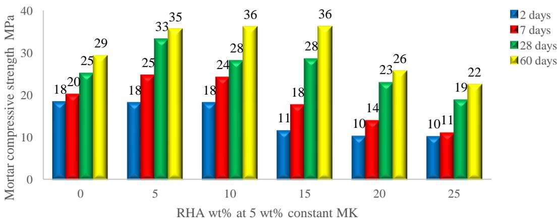
Figure 15 – Effect of RHA content at constant 5 wt% MK on compressive strength of blends and OPC mortars
