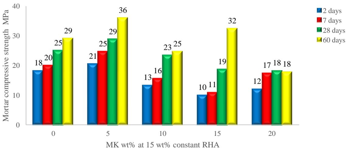
Figure 13 – Effect of MK content on mortar strength of blends at constant 15 wt% RHA and OPC
