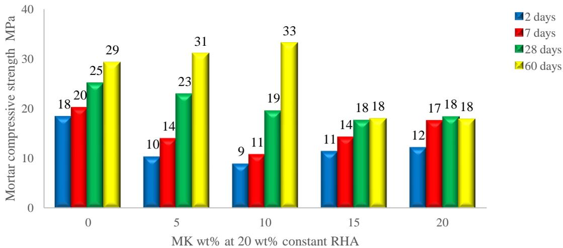
Figure 14 – Effect of MK content on mortar strength of blends at constant 20 wt% RHA and OPC
