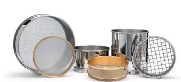
Figure 2 – A set of sieves for the Sieve Analysis Test
