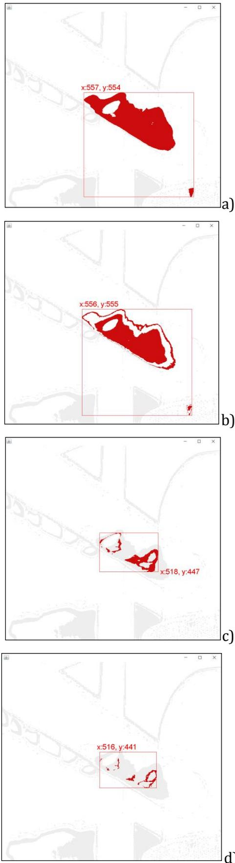
Figure 7 – Analysis of a damaged pipeline with different shades of damage colour: a) – red = 100 and green = 70 and blue = 70, b) – red = 150 and green = 100 and blue = 100, c) – red = 200 and green = 50 and blue = 50, d) – red = 210 and green = 50 and blue = 50
