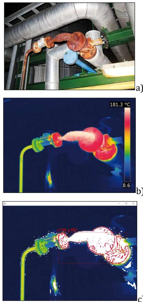
Figure 1 – The process of analyzing a damaged pipeline: a) – the original image of the pipeline [24], b) – the thermal image of the pipeline [25], c) – the processed image of the pipeline
