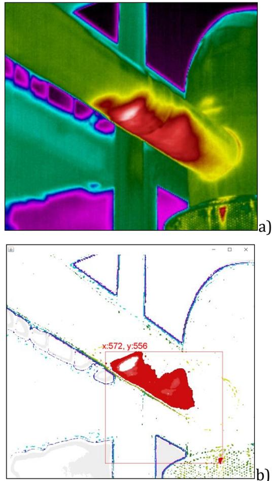
Figure 6 – Analysis of the damaged pipeline: a) – the thermal image of the pipeline [30], b) – the processed image of the pipeline
