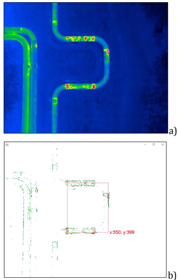
Figure 3 – A damaged pipeline from the aerial survey:
