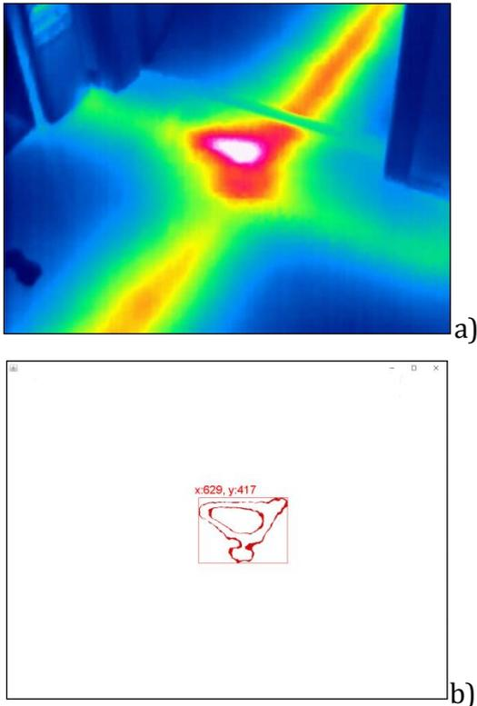
Figure 4 – A damaged pipeline at the junction of several pipes: a) – thermal imaging image of the pipeline [28], b) – the processed image of the pipeline
