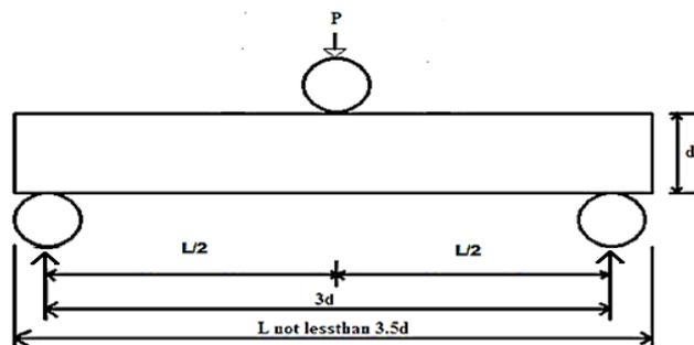
Figure 1 – Loading Arrangement for Flexural Strength Test Specimen (Three Point Bending)
