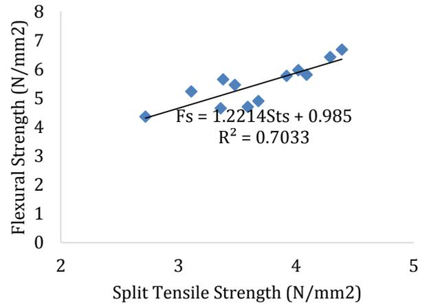
Figure 9 – Relationship between Flexural and Split Tensile Strength of Concrete Containing WCWF
