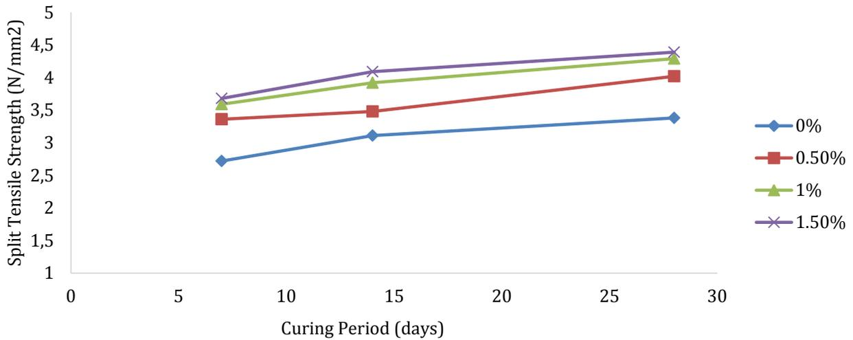
Figure 6 – Split Tensile Strength of Concrete Containing WCWF
