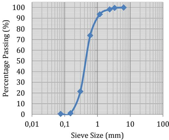
Figure 2 – Grading curve for fine aggregate
