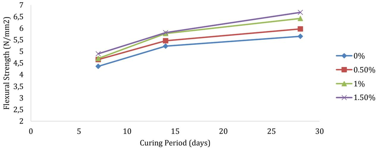
Figure 5 – Flexural Strength of Concrete Containing WCWF
