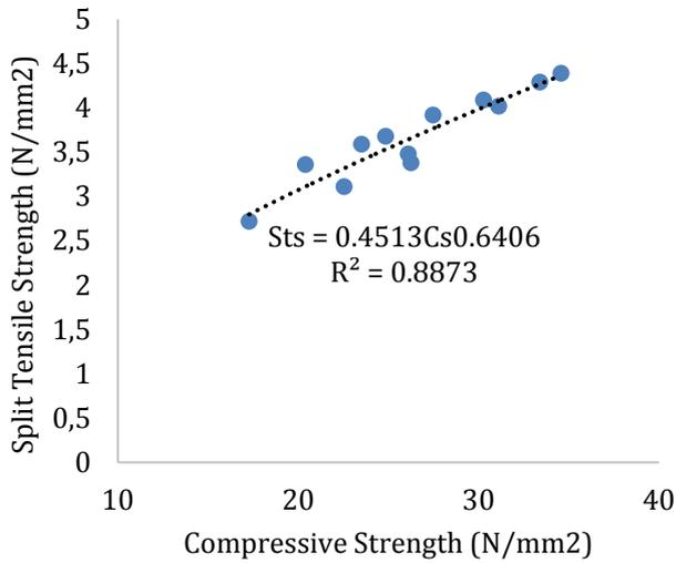
Figure 8 – Relationship between Split Tensile and Compressive Strength of Concrete Containing WCWF
