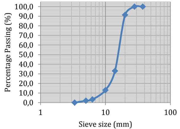
Figure 3 – Grading Curve for Coarse Aggregate
