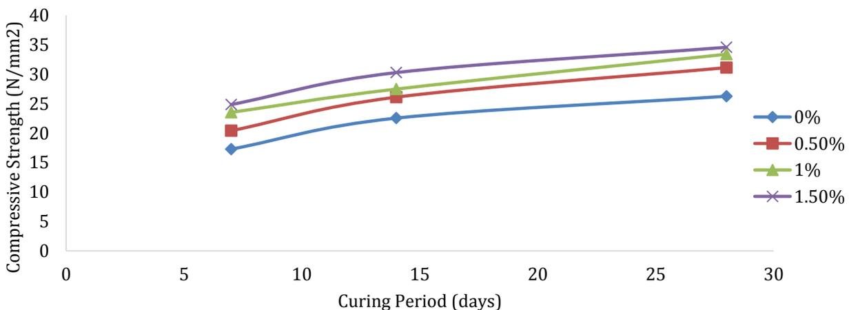
Figure 4 – Compressive Strength of Concrete Containing WCWF
