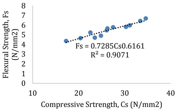
Figure 7 – Relationship between Flexural and Compressive Strength of Concrete Containing WCWF
